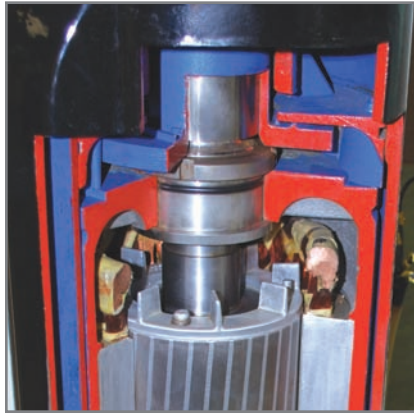
A cutaway of a Wilo pump
